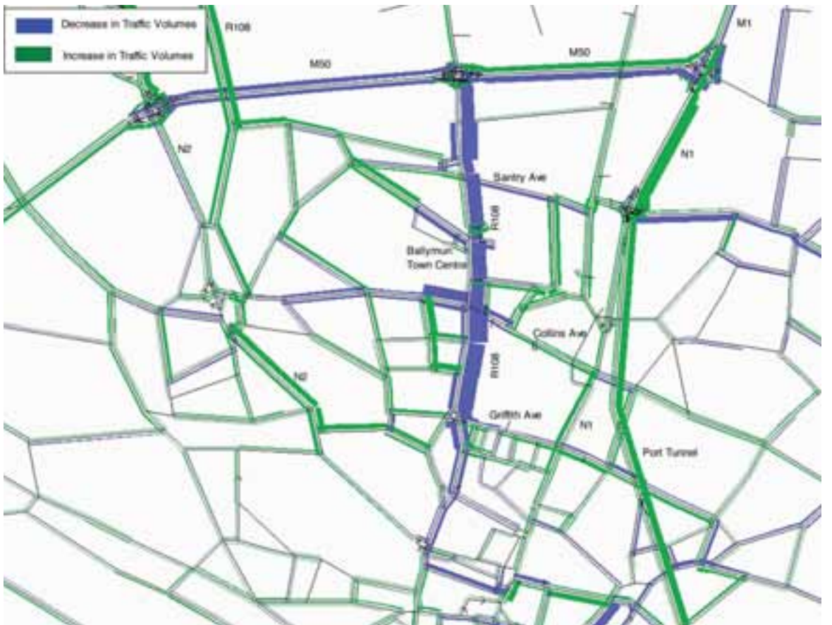
Figure 7.5 Traffic flow changes – do- minimum vs. do-something 2011 (Ballymun/ Glasnevin/ Finglas/ Drumcondra areas)
